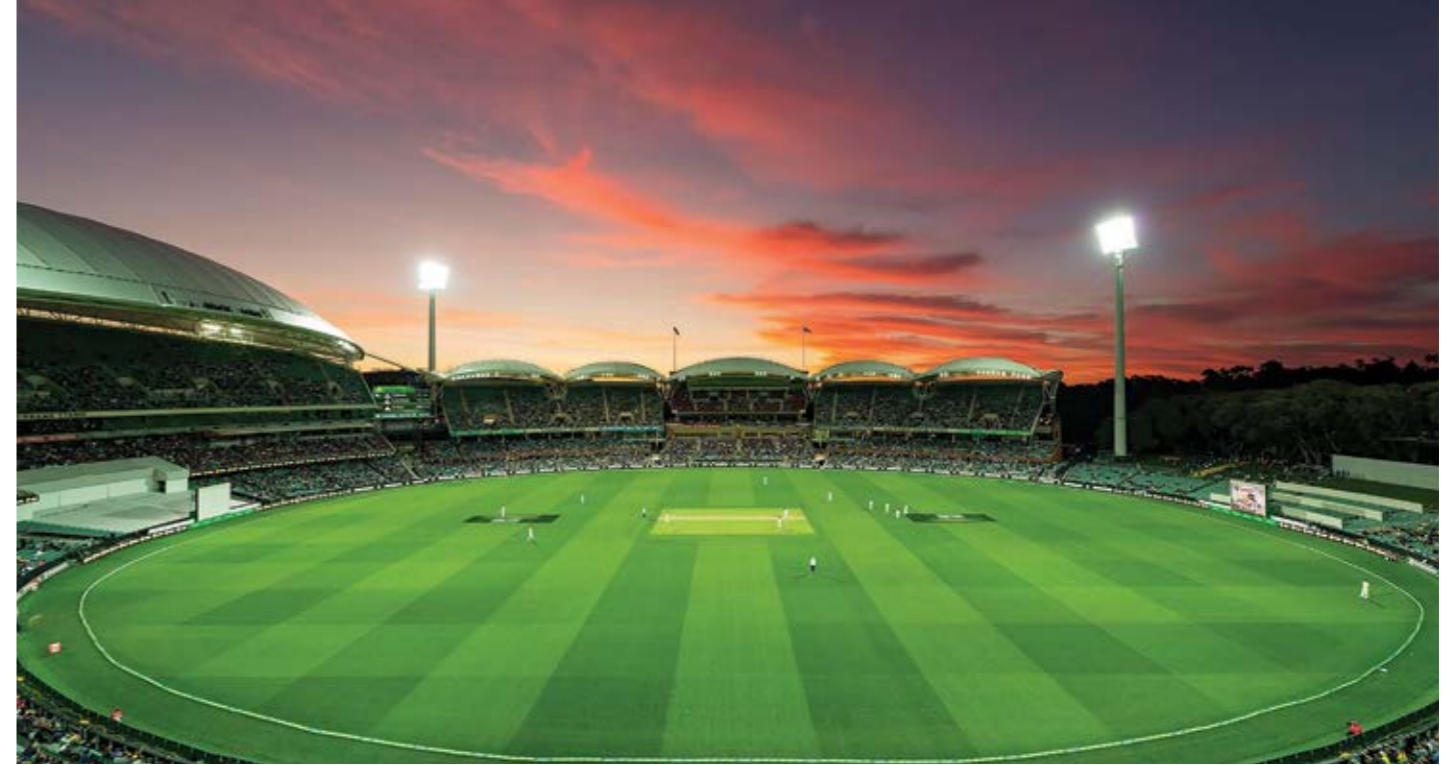
Adelaide Oval's outstanding lighting for night cricket still comes mainly from metal halide lamps.
