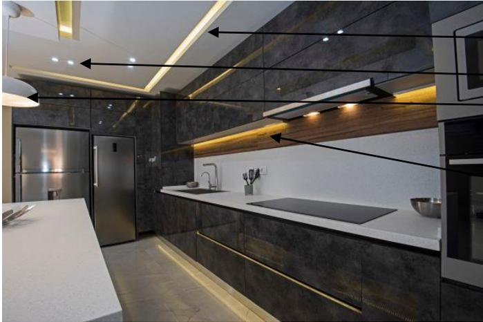
Downlight and pendant fixtures provide general and task illumination. LED strip lighting is used to accentuate architectural features and increase visual interest.
