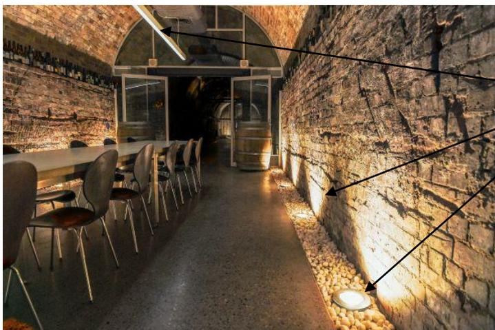
A linear lighting fixture provides task illumination over the dining table. Up lighting around the perimeter of the room is used to graze/wash the walls with light to highlight the wall texture and fill the room with gentle diffuse light.
