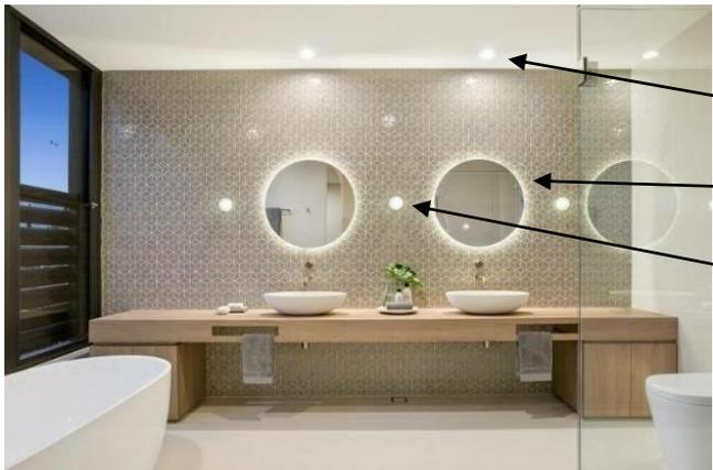
This bathroom uses down lights to provide general and task illumination, diffuse wall lights to light faces while using the mirrors and LED strip behind the mirrors to create visual interest.
